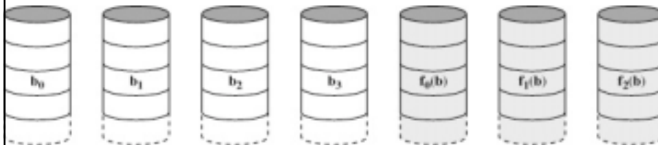
c) RAID 2 (redundancy through Hamming code)
