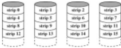
(a) RAID 0 (non-redundant)
